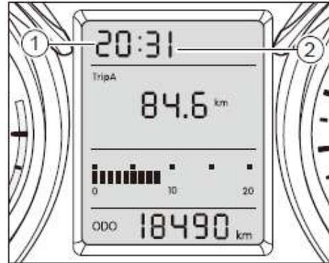
When the ignition switch is at the position “ON”, on the trip information interface, if you press down and hold the button INFO and the button RESET, the hour ① will flash; if you press the button INFO and the button RESET again, the hour will be set (whenever the button is shortly pressed, the value will increased by 1; if the button is pressed down and hold, the value will increase continuously).
